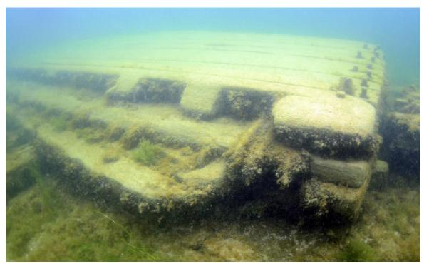
Figure 17. Grape Shot's centerboard and centerboard trunk
